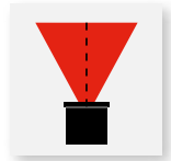
Reflector 20% scat Y10% = 2 x 22,6° Y50% = 2 x 13°
