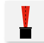
Reflector 0% scat Y10% = 2 x 6,6° Y50% = 2 x 3,6°
