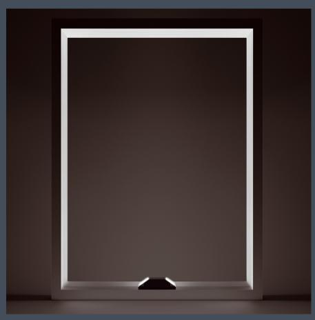
Arclight is a luminaire for the accent lighting of window reveals. The light from 2 LEDs is directed from the opposite sides of the luminaire, via specially developed reflectors, onto the widow reveal. The result is a uniform arc of light. A complete window reveal can be illuminated using just one luminaire.
