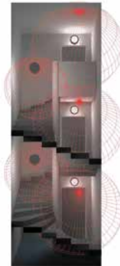
Spiral stairway stairwell dimensions: 2.7 m × 2.7 m, ceiling height 2.5 m
