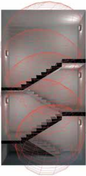
Rectangular stairway stairwell dimensions: 2.6 m × 4.3 m, ceiling height 2.5 m
