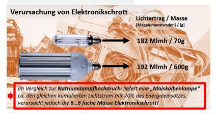
Compared to a high-pressure sodium vapor lamp, a corncob lamp delivers approximately the same cumulative luminous flux with 70% of the energy input, but causes 6 to 8 times the amount of electronic scrap!
