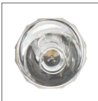
Reflector rotationally symmetric without facets (unscattered), very narrow distribution of 7^\circ ( Y_{50\%} = 2 \times 3,6^\circ )
