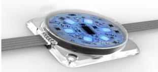
GRAPH-i-DOT is an ultra compact module fitted with 6 mid-power full colour LEDs for ultra luminous spot light performances. Graph-i-Dot is the ideal solution to screen low resolution video files and graphic patterns. Graph-i-Dot can accept, via DMX interface, any graphic, video or still image coming from a DVI media server and the configuration system can then store and trigger the show to a striking visual effect. The IP68 weather protection rating allows under water use.
