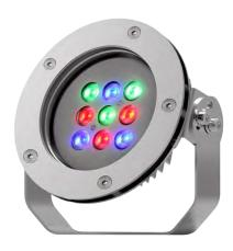
Small-size fountains and waterfalls, as well as reflecting pools, are the ideal applications for the compact marine-grade MINI WATERLED, whose heavy-duty AISI 316L stainless steel body hosts nine high power LEDs. The superior lumens life assisted by the on-board electronic thermal management exceeds the industry standards lifetime and the certified IP68 Class III rating defines the virtually maintenance free performance.
