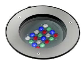
DUNE MK2, with its IP67 rating, is a highly performing LED light fitting specifically designed for exterior recessed applications. The 2000 Kg deadweight load capacity makes this fixture suitable for ground mounting applications even in vehicular areas. DUNE MK2 also features beam angle orientation adjustment.
