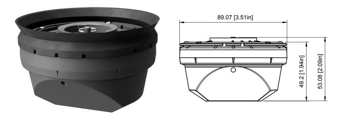
Comlight Eagle Eye Zhaga is a motion detection light controller for luminaires complying with Zhaga Book 18 specification and SR (System Ready) concept. The sensor is designed according to Dali-2 (IEC62386), part 303 Occupancy sensor as a D4i Type B device, in addition to automatically taking role as a Type A controller device if no other controller is present.
