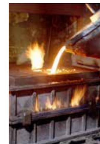
Models created by Neri allowed to cast all the components of the posts. This operation was quite difficult and delicate, as the models had to be made of various parts because of the rich decorations of the posts.
