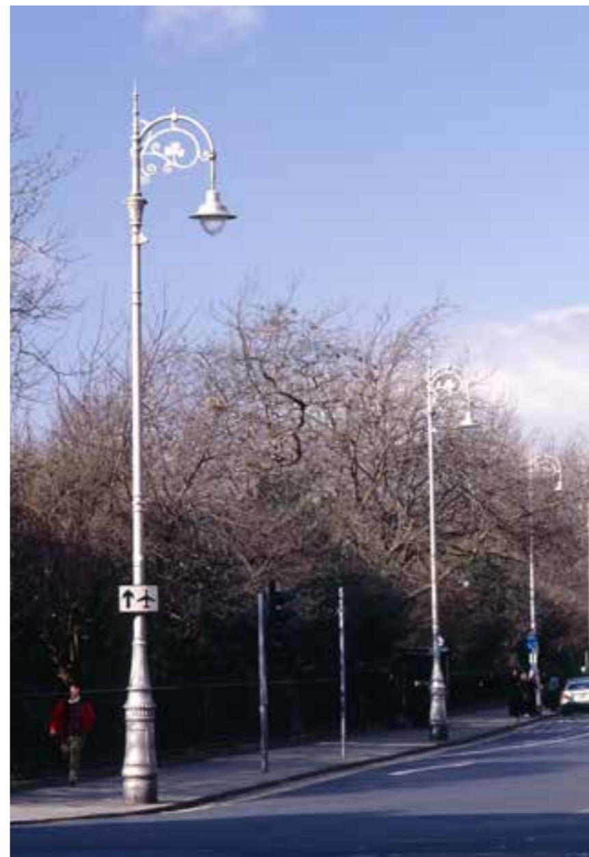
The post with swan neck top which was reproduced for some areas of the city is particularly beautiful and impressive. The swan neck top shows an Irish shamrock; this post is fitted with Light 22 luminaire.
