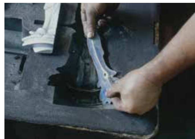
Models created by Neri allowed to cast all the components of the posts. This operation was quite difficult and delicate, as the models had to be made of various parts because of the rich decorations of the posts.
