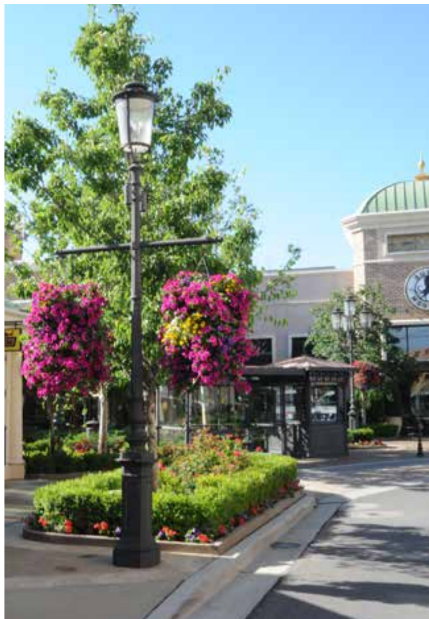
Special posts were designed for the Station Park malls in Farmington and The Village in Meridian (U.S.), they include a flower box support with integrated automatic irrigation system, to solve the serious problem of flower maintenance. Special modified bicycle racks were installed in both malls.
