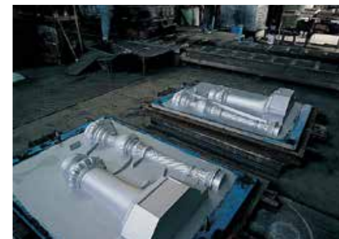
Models created by Neri allowed to cast all the components of the posts. This operation was quite difficult and delicate, as the models had to be made of various parts because of the rich decorations of the posts.
